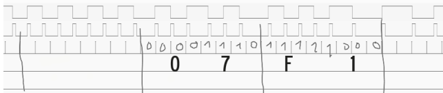
Figure 7: Extract of bitstream showing identification mark and track number
